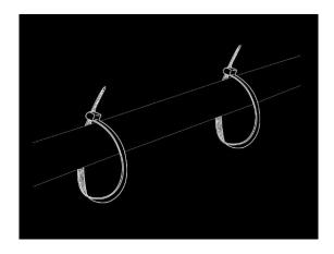
2. Place the Monitor on the pipe so that you can see the top of the Monitor easily. There are two LED lights on the top of the Monitor that need to be visible so that the
