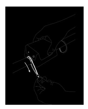
4. Repeat step #3 with the other zip-tie. Once the Monitor is secured, tighten each zip-tie so that the Monitor is snug against the pipe. **Do not attempt to twist or slide** the Monitor once it has been zip-tied to the pipe. This can cause damage to the sensor pads. If you damage the sensor pads during this process, <u>click here</u> to read how to replace the pads.
