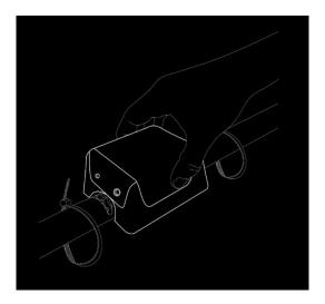
3. Hold the Monitor in place with one hand and tighten a zip-tie around one of the zip-tie channels with the other hand by pulling on the end of the zip-tie, as shown below. By tightening the zip-tie over the zip-tie channels, you are securing the Monitor to the pipe.
