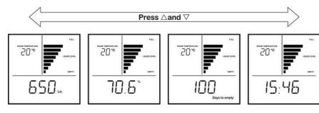
For approximately 1 week after the monitor is installed, it collects data so that the 'Average per Day' value may be calculated. During this period the screen will flash '---' when showing 'Days to Empty' – this is shown as a red circle in the diagram to the right.
